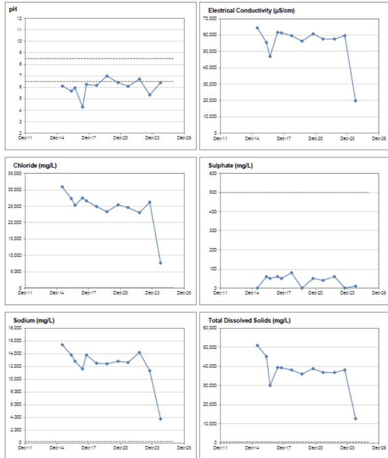
GROUNDWATER TREND CHARTS - MONITORING WELL TH15-7 2024 SOIL AND GROUNDWATER ASSESSMENT ACTIVITIES TOWN OF SLAVE LAKE - PUBLIC WORKS YARD 1009 - 7 STREET NE, SLAVE LAKE, AB
