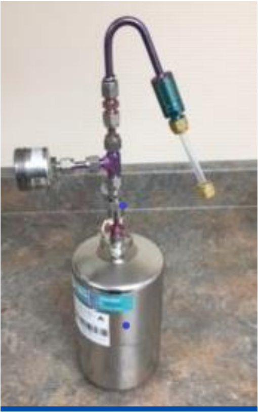
1.4L Silonite canister with short-term grab sampler or long-term TWA
