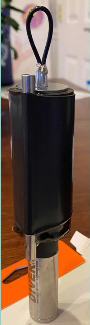
LNAPL monitoring configuration shown. Minimal LNAPL thickness required for fluid interface transducer to maintain proper buoyancy
