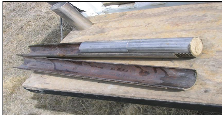
California Split Spoon Core Barrel, Stainless Steel Sleeves and Hollow Stem Auger
