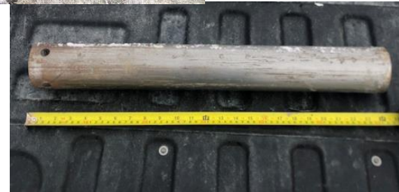
Shelby Tube/ 3' Long Agriculture Core Barrel
