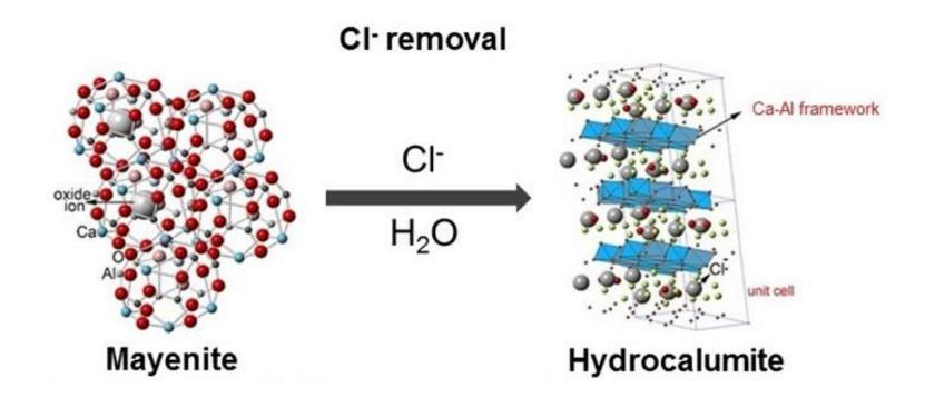
Cl<sup>-</sup> is removed from the aqueous phase and trapped in the mineral phase through the mayenite-to-hydrocalumite mineral phase change
