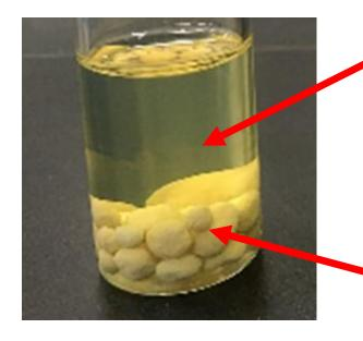
Nonaqueous Phase Liquid (free phase diesel)
