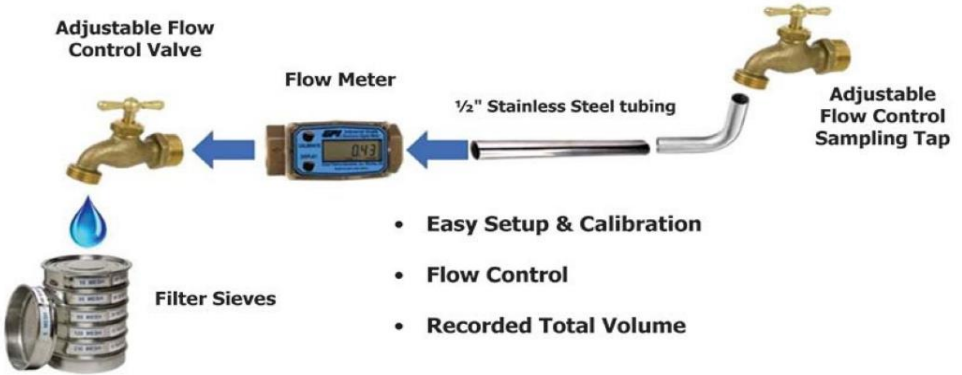
FIG. 2 Water Sampling Apparatus for Pressurized Systems
