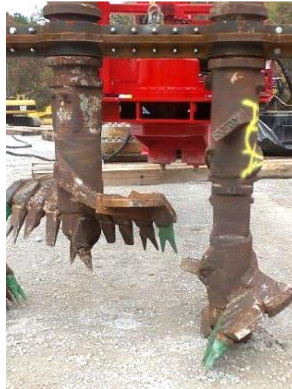
Multi auger drill
