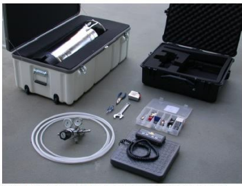
Contents of bioaugmentation field injection kit, includes vessel in over pack, hose, regulator, spare fittings and miscellaneous tools
