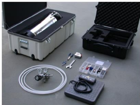
Contents of bioremediation field injection kit, includes vessel in over pack, hose, regulator, scale fittings and miscellaneous tools
