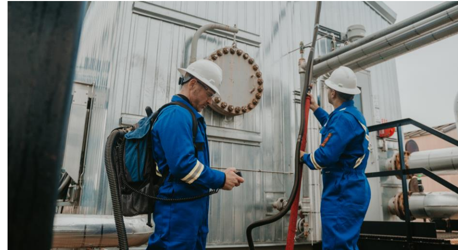
Flow Rate Quantification Bacharach Hi Flow Sampler
