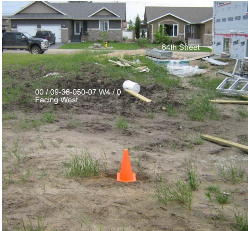
Well location with surface casing below grade and apparently stressed vegetation when first found by the OWA in 2013
