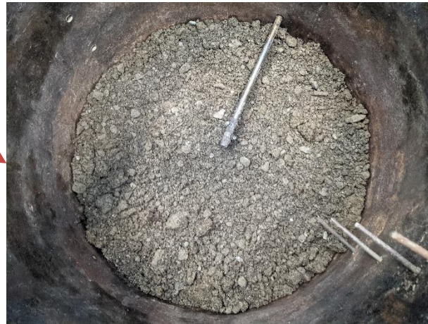
PFAS-Impacted Field Soil + 40 g/kg GAC + 10 g/kg CaO
