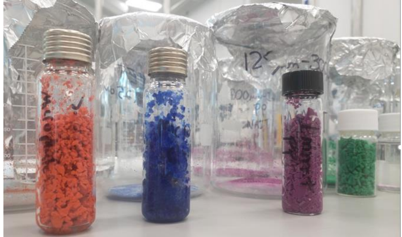
Image: Microplastic standards created from common plastics found in the lab (PVC, PET, PE, PP)
