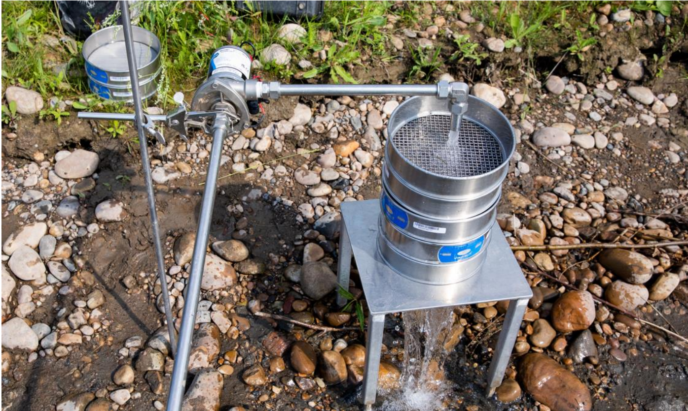
Images: ASTM pumping system with cascade sieves for microplastic sampling
