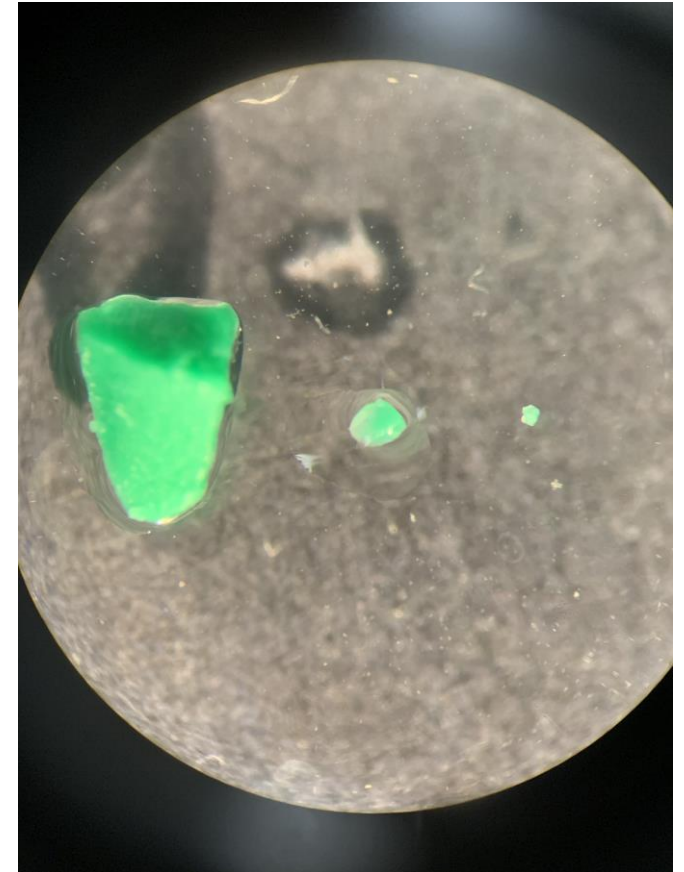
Image: Lab Created Polypropylene microplastics 1mm-100µm
