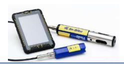
The Aqua TROLL 500 is a multiparameter sonde for pH/ORP/EC/RDO/Turbidity/Temp (includes Flow Cell). Connects to a tablet or Android smartphone, allowing you to collect and analyze data.
