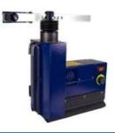
Portable, electric or gas powered device used to automate the Inertial Pump.
