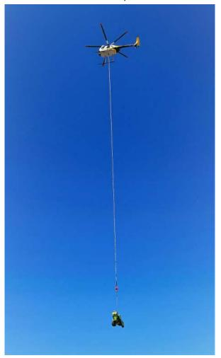
Can be flown in 2 separate lifts by a MD500 or 1 lift with an AStar AS350B2/B3
