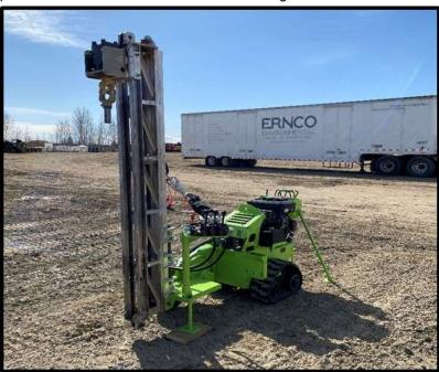
Mobile drill that can move around a site without UTV or Helicopter support.
