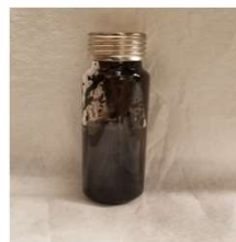
Headspace vial – direct GC analysis (1:1)
