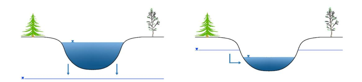
Groundwater Recharge (losing stream) Groundwater Discharge (gaining stream)
