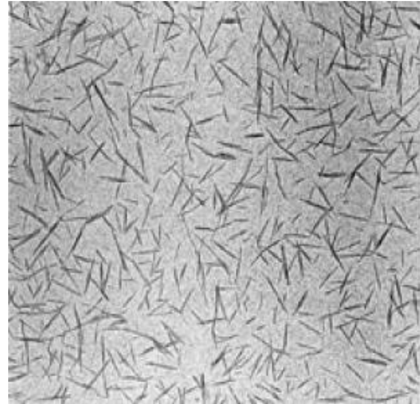
Particle diameter: 5-15nm Particle length: 100-200nm
