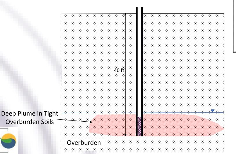
Needed backfill material that can be drilled through while providing sufficient injection resistance?
