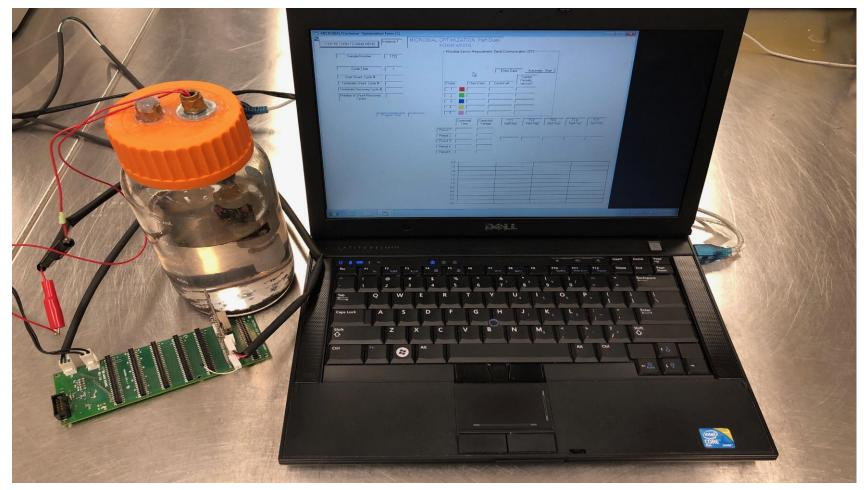
Circuit closes to expel deposited electrons and then opens to measure re-deposition in mV
