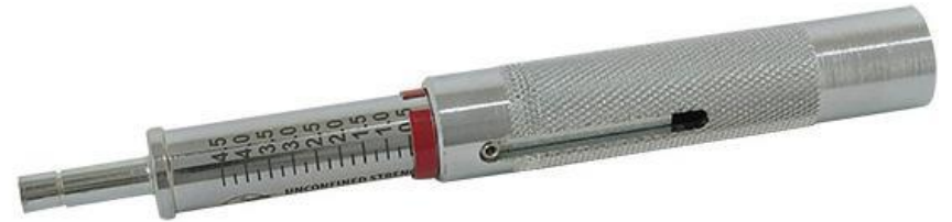
Pocket Penetrometer for Field measurement of UCS
