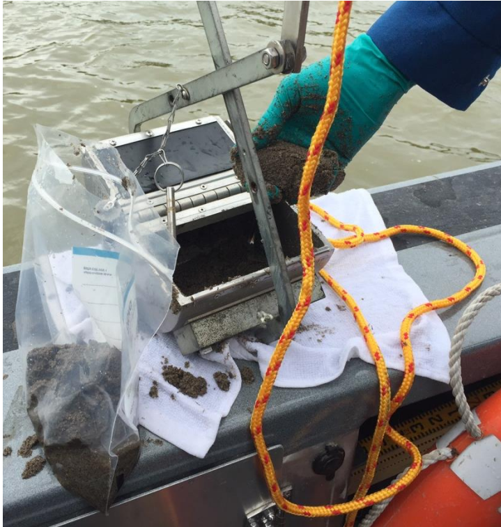
Sediment Sample Collection using a Ponar Dredge (Left)
