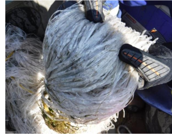
Visual Hydrocarbon Deposition on SODD
