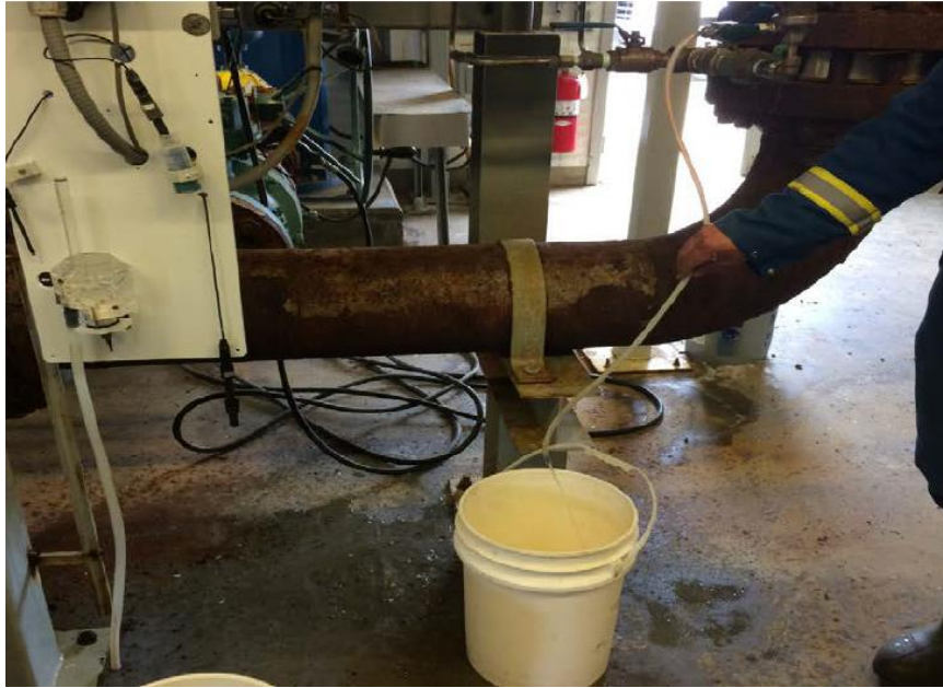
Infiltration Gallery Well Samples Being Collected into a Clean Bucket
