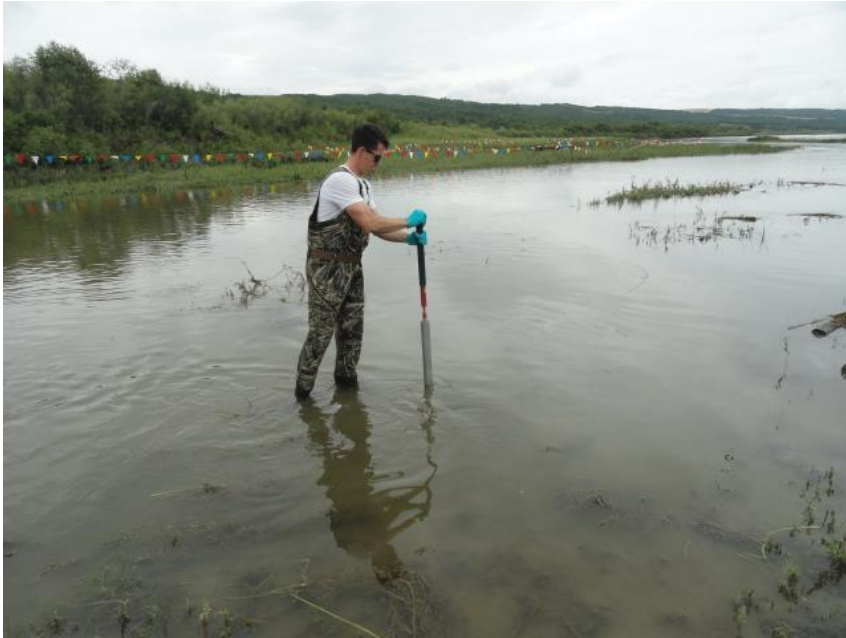
Sediment Core Collection using an AMS Sediment Sampler (Left)
