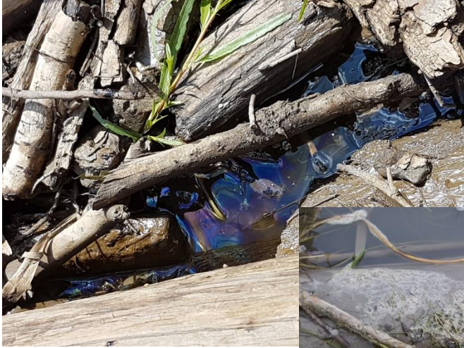
Free-phase hydrocarbon, sheen and foam
