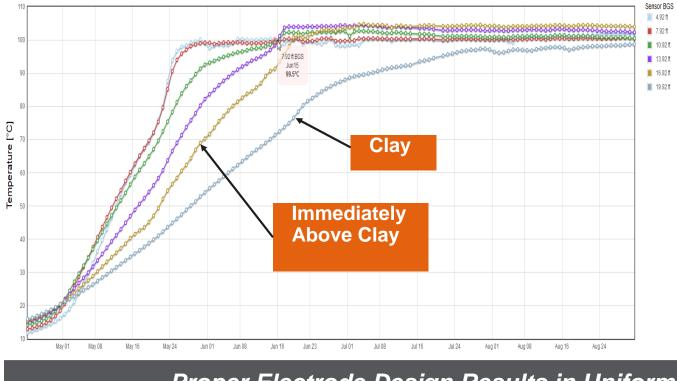
Proper Electrode Design Results in Uniform Heating
