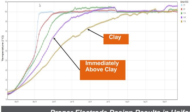
Proper Electrode Design Results in Uniform Heating
