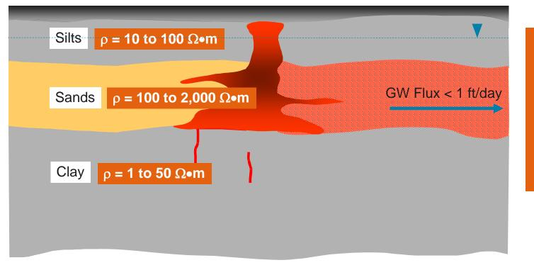
CVOC Source Zone to be Treated With Electrical Resistance Heating (ERH)
