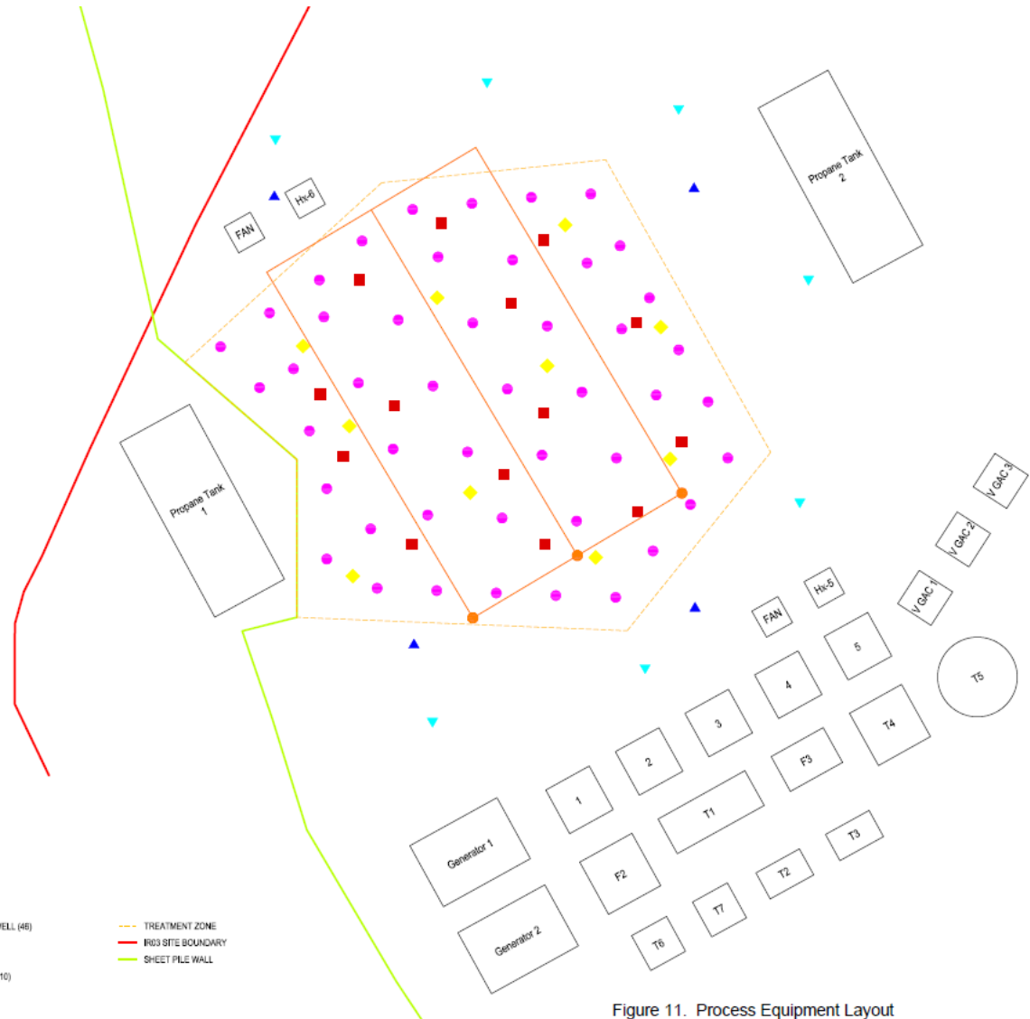
Figure 11. Process Equipment Layout
