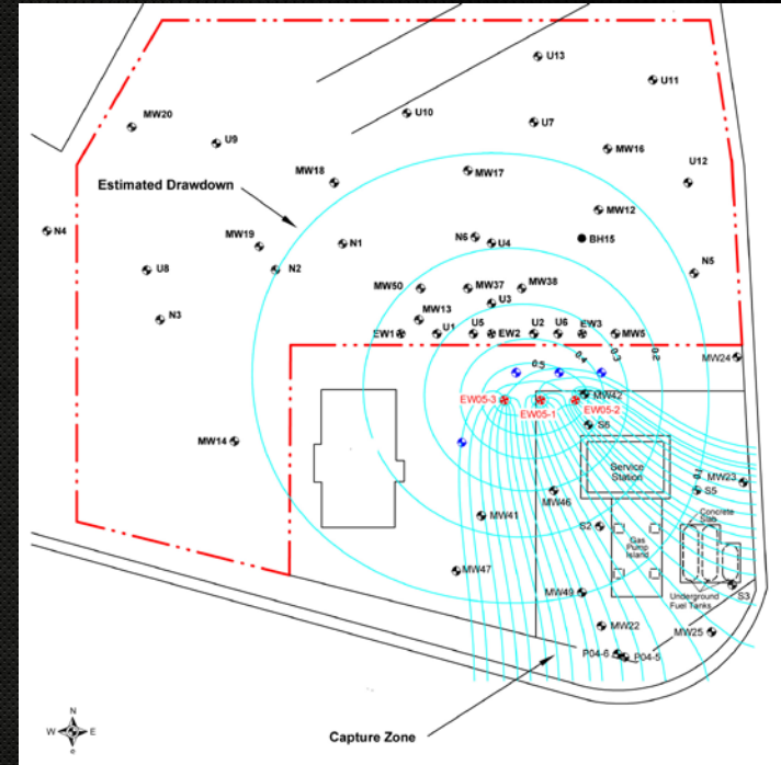
Dual Phase Extraction System Without Overlapping ROI
