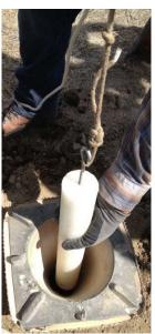
Sustained-release persulfate is a NaS2O<sub>8</sub>-based product dispersed in a solid paraffin wax matrix (~80% w/w)
