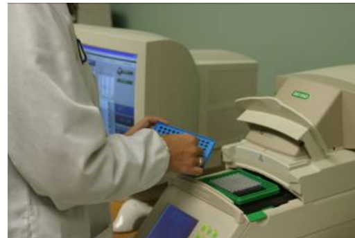
6) PCR amplify specific genes with targeted primers in qPCR Machine
