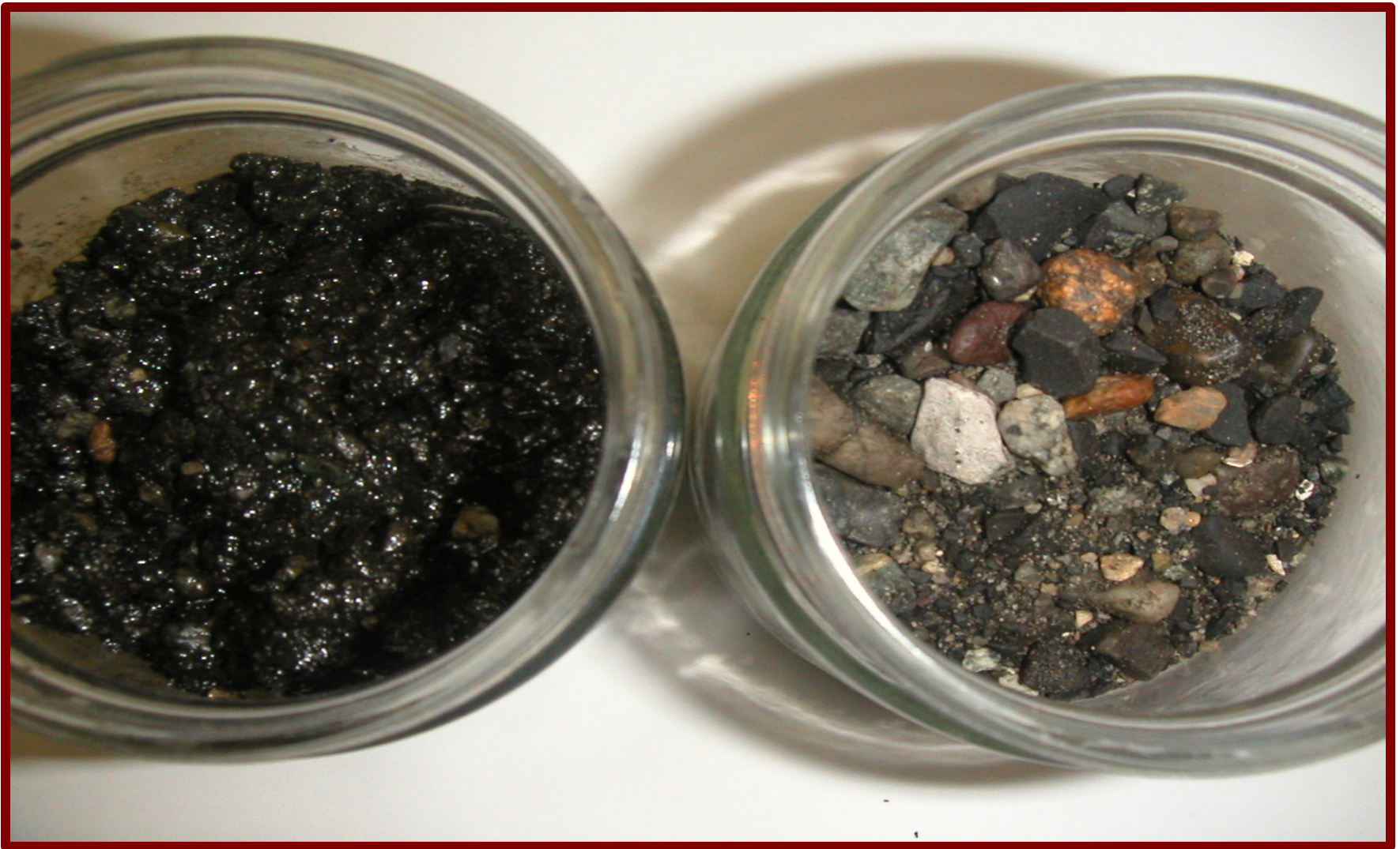
Pre and post Ivey-sol Surfactant washed solids impacted with heavy-end petroleum hydrocarbons
