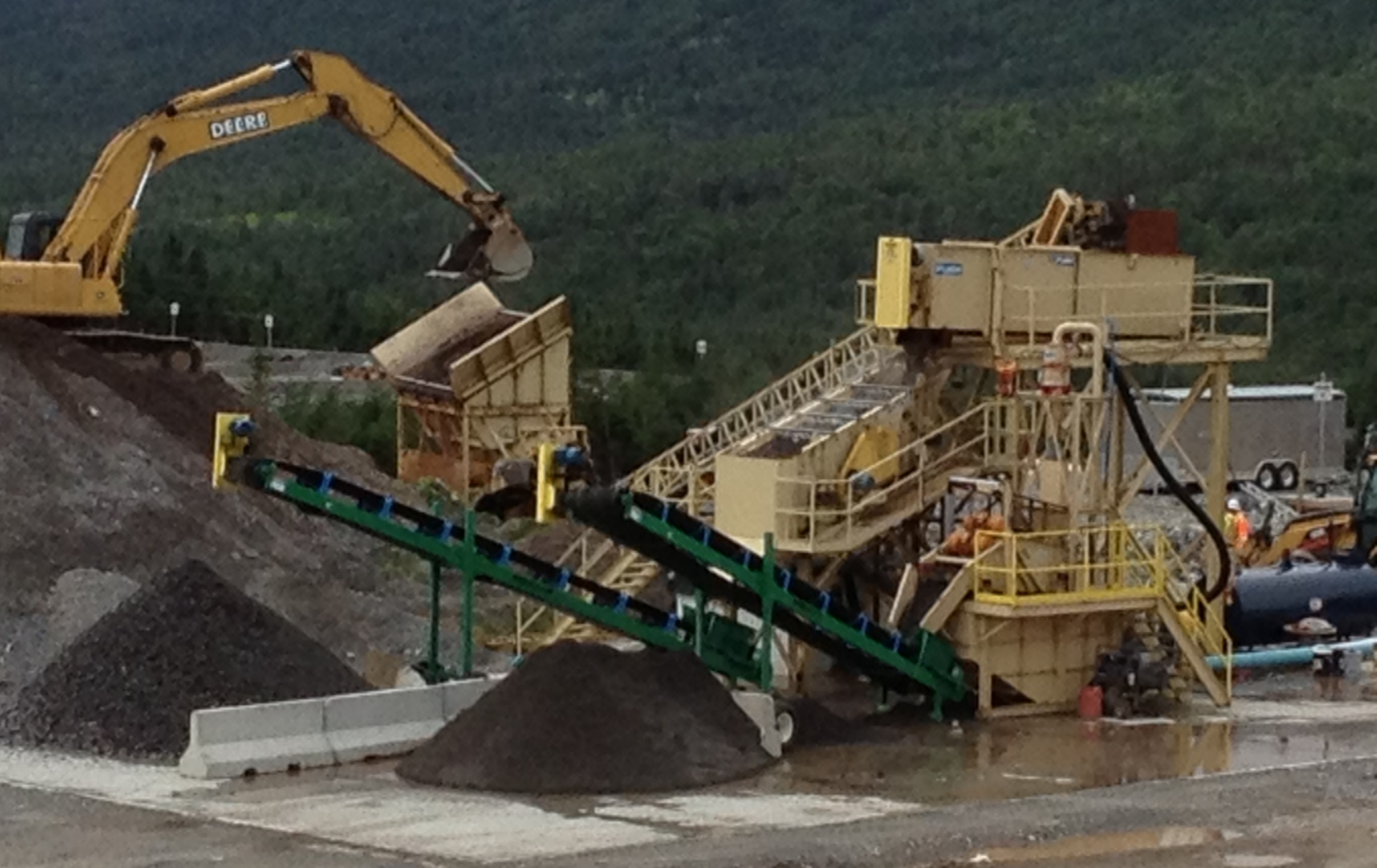
CONTINUOUS SOIL WASHING SYSTEM 50 TO 150 TONS/HOUR
