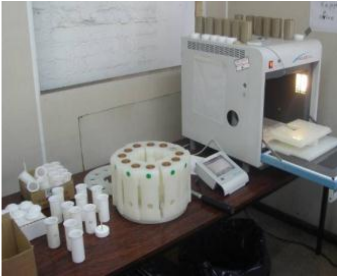
On-site laboratory analysis of pore water concentrations using Microwave Assisted Extraction (MAE)
