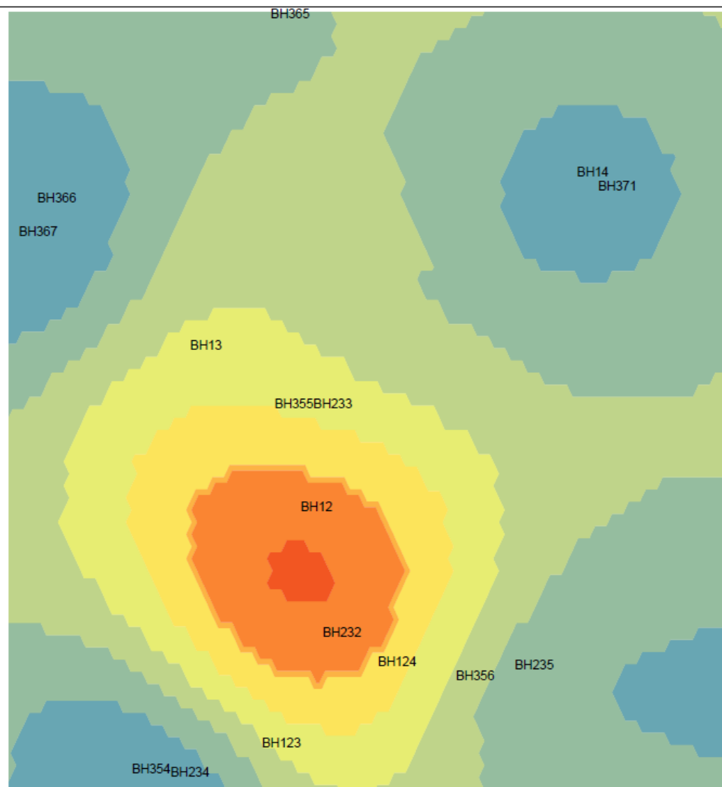
Chloride prediction map at 10 feet depth, Quantile 75%
