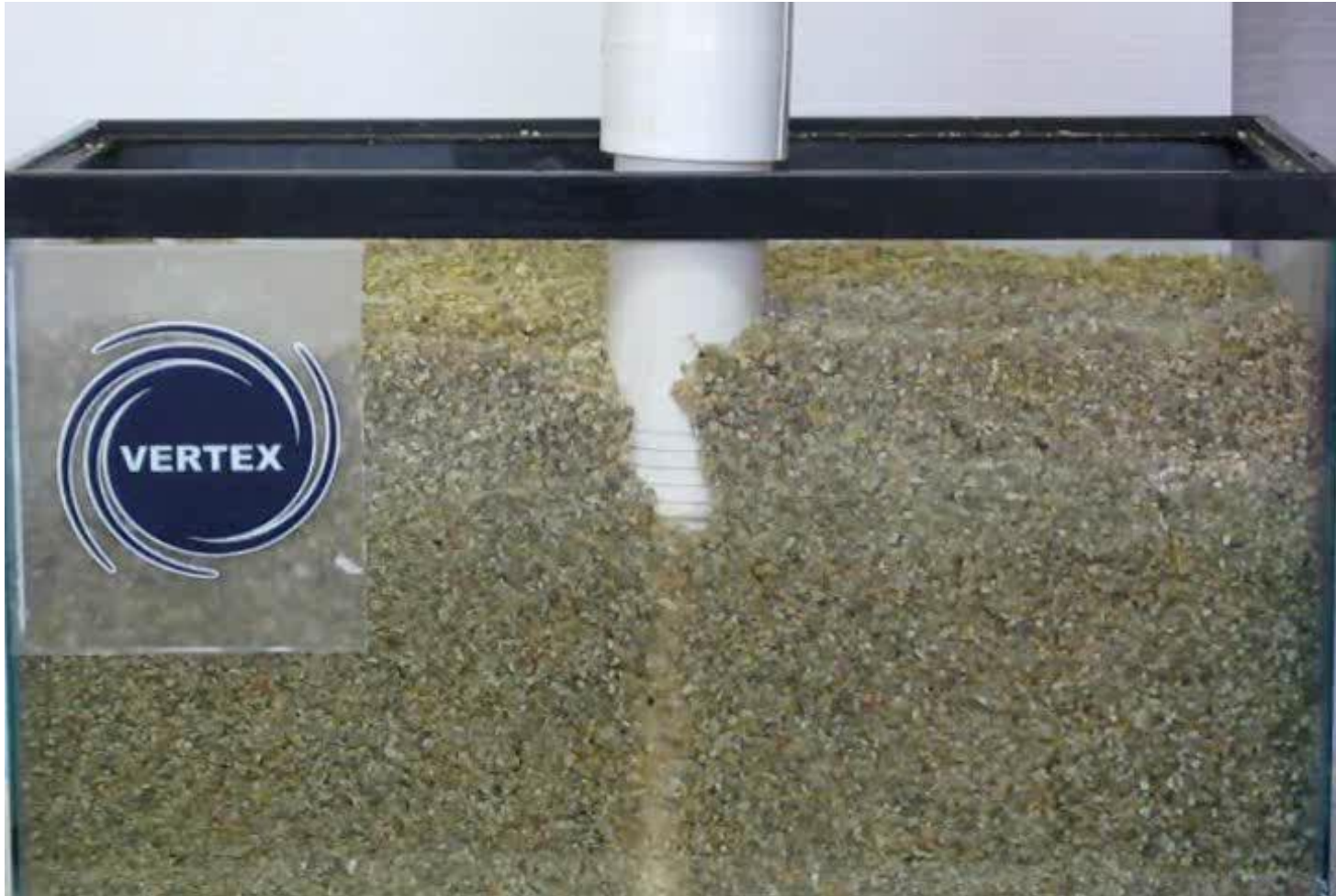
Injection Well, Experiment #1 2" diameter PVC Slot 10 Well, screened to bottom of tank Flow = 4.5 lpm
