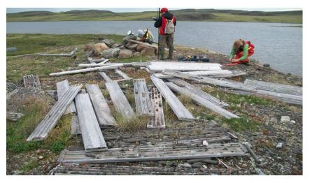
Drill core boxes with drill core
