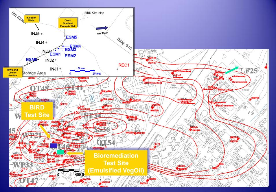
Dover AFB TCE plume, test site location and injection layout schematic
