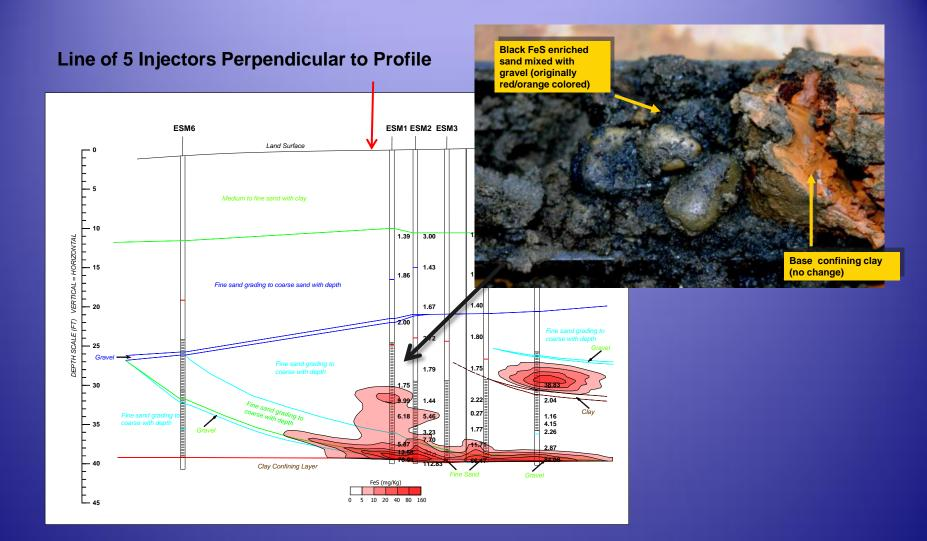
Profile of mineral FeS development (mg/Kg as S) and example photo of sediment core with FeS.
