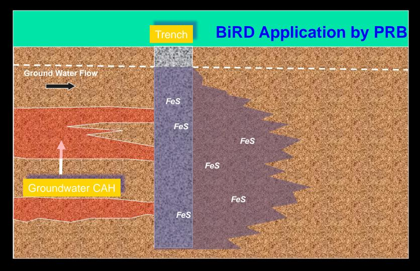
Solid reactants form solid FeS so is mostly "invisible" to aqueous monitoring. FeS forms in the trench and down-flow gradient
