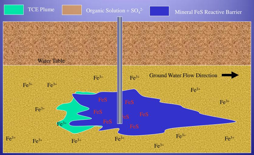
FeS forms a permeable reactive zone into which aqueous CAHs may flow. Dechlorination is complete and dechlorinated products are mineralized to CO2.
