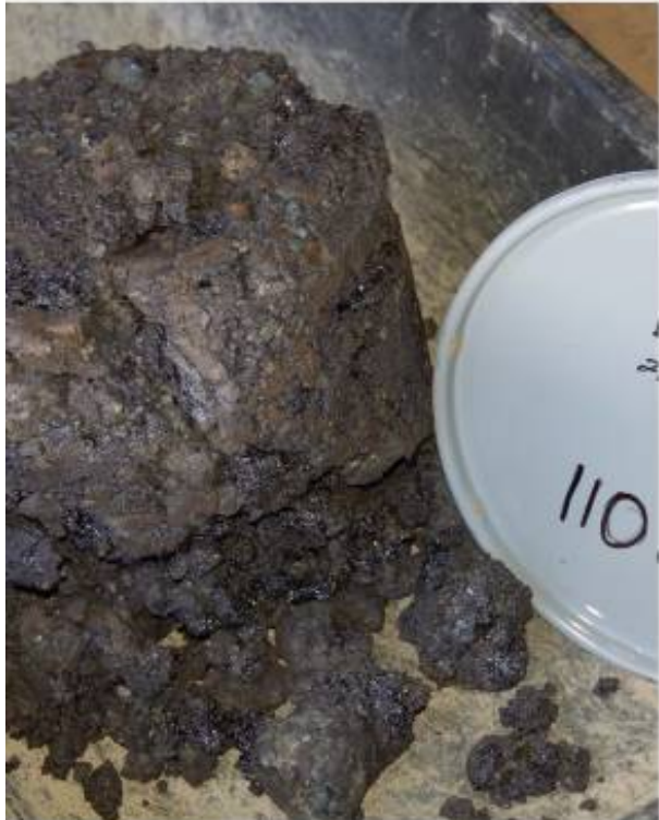
Oily Soil Before S/S
