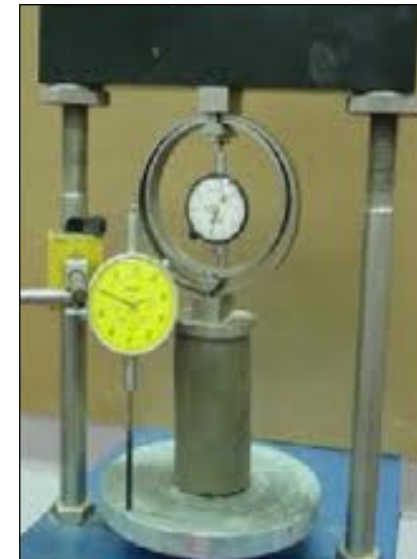
ASTM D1633: UCS for soil-cement cylinders
