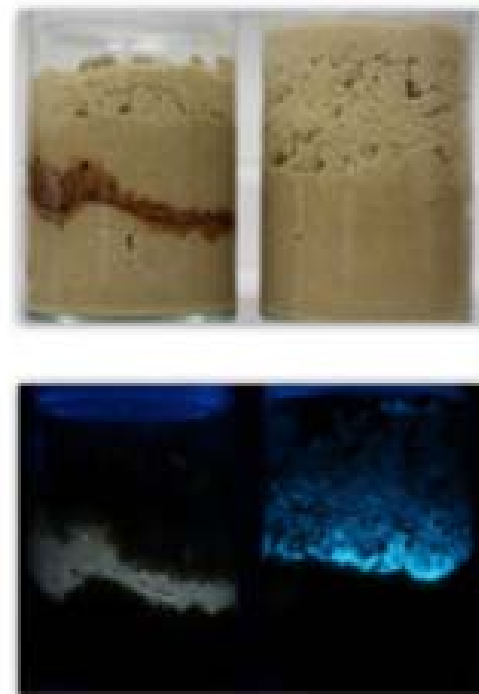
Photographs of crude oil (left) and diesel fuel (right) on water-saturated sand under room light (top) and long wavelength ultraviolet lamp excitation (bottom).
