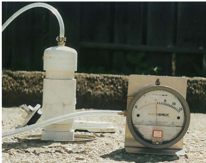
Typical well headspace vacuum monitoring equipment.
