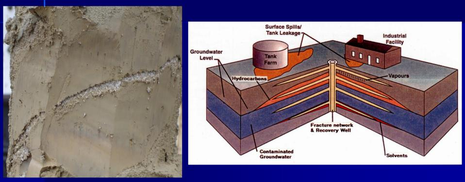
Fracturing is a process in which fluid is applied to a soil or rock mass until failure of the soil or rock occurs, which results in a tensile parting (i.e. fracture)
