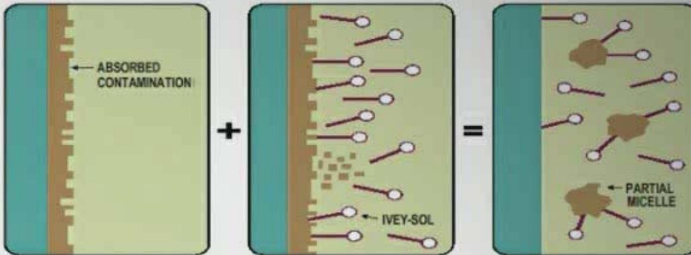
Ivey-sol<sup>®</sup> shown desorbing contamination off a surface. Once liberated the desorbed contaminants have increased 'Availability' for improving the associated in-situ or ex-situ remediation method being employed.
