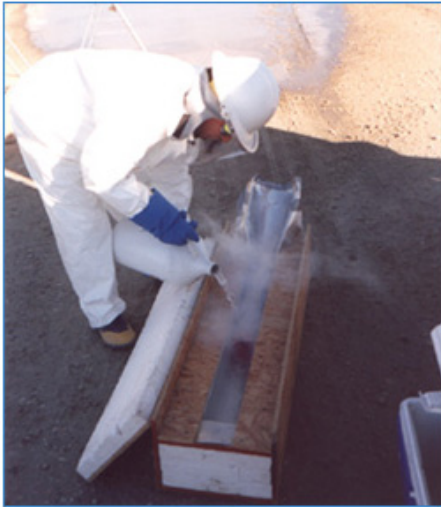
Preserving core using Liquid Nitrogen
