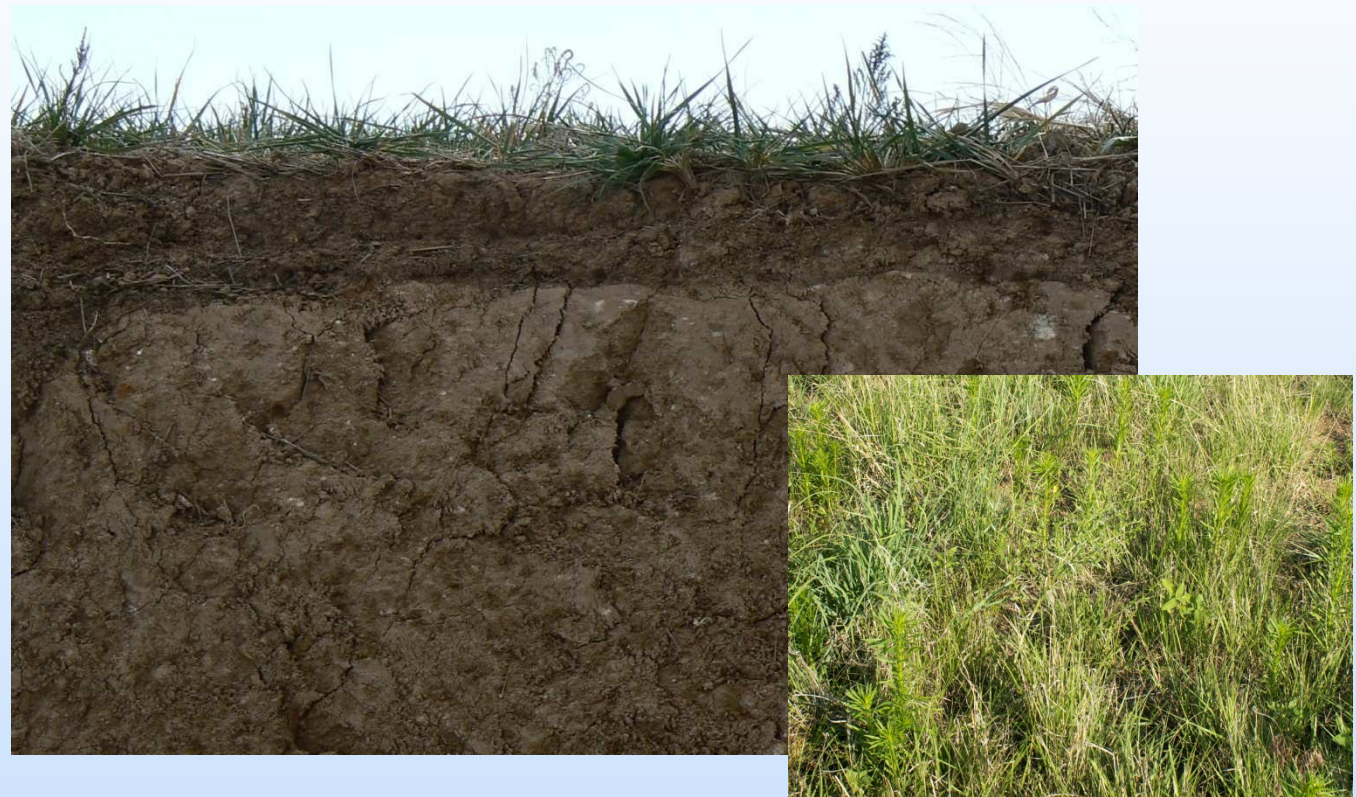
Cross section of the Shell RCRA-Equivalent Cover. Progress of vegetation after one growing season. (EPA field oversight photograph)
