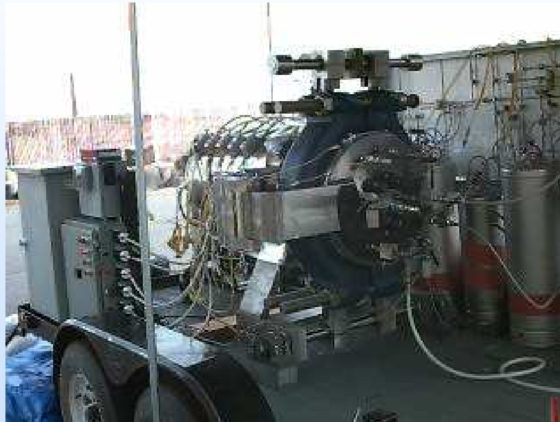
The Explosive Destruction System (B.L. Haroldsen, J.H. Stofleth, and T.J. Shepodd)
