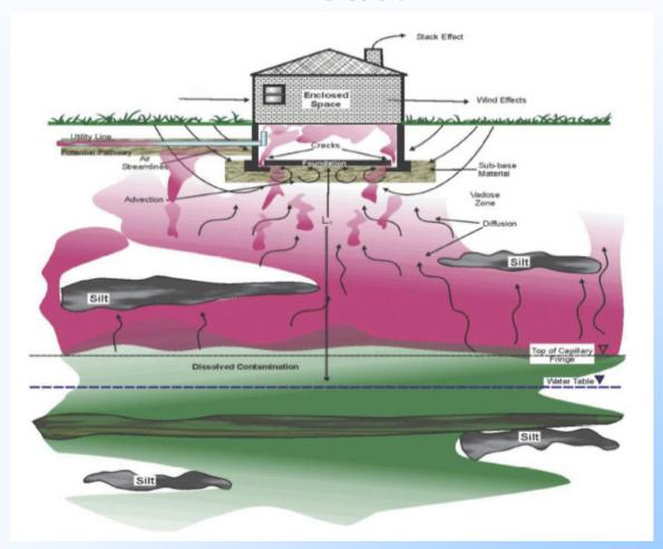
Example of a Conceptual Site Model for Vapour Intrusion into a Residential Building (adapted from US EPA, 2002)
