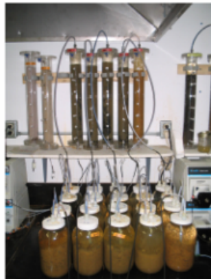
Photograph 1. EHC treatment columns with downstream attenuation jars.
