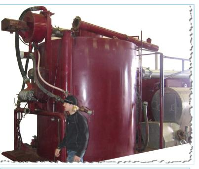
The exhaust gas from the chamber is transferred to the tank to condensed into a recyclable liquid.
