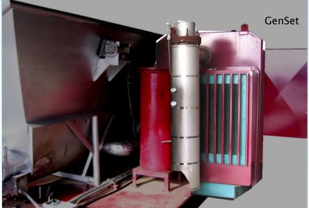
Independently controlled electric elements and hot exhaust gases from the self contained electric generation unit.
