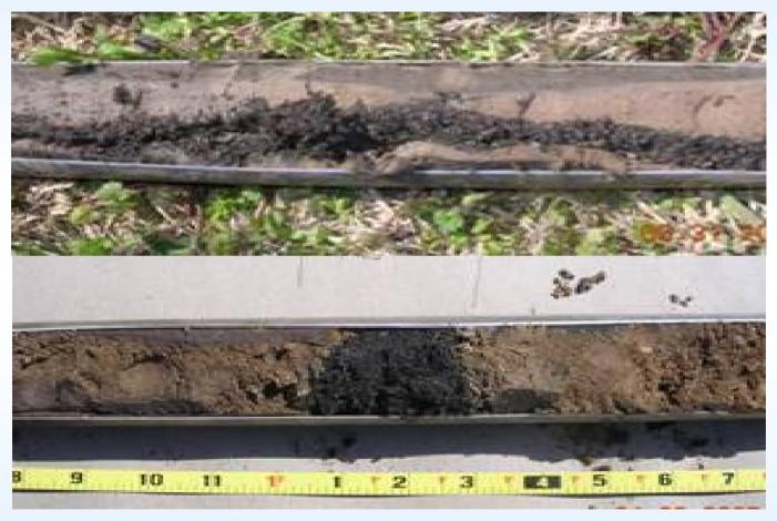
Soil cores obtained at the beginning of the installation to verify radius of influence and determine injection spacing
