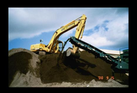
Contaminated media can be processed in a dry non-monolithic form to minimize disposal costs or with higher moisture content to minimize dust and enhance material handling characteristics
