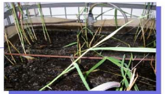
GRAVEL (SUBSTRATE) COVERED BY PEAT
