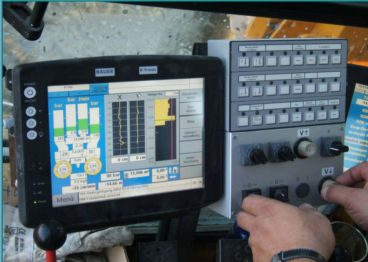
B-TRONIC touch screen in operators cabin
