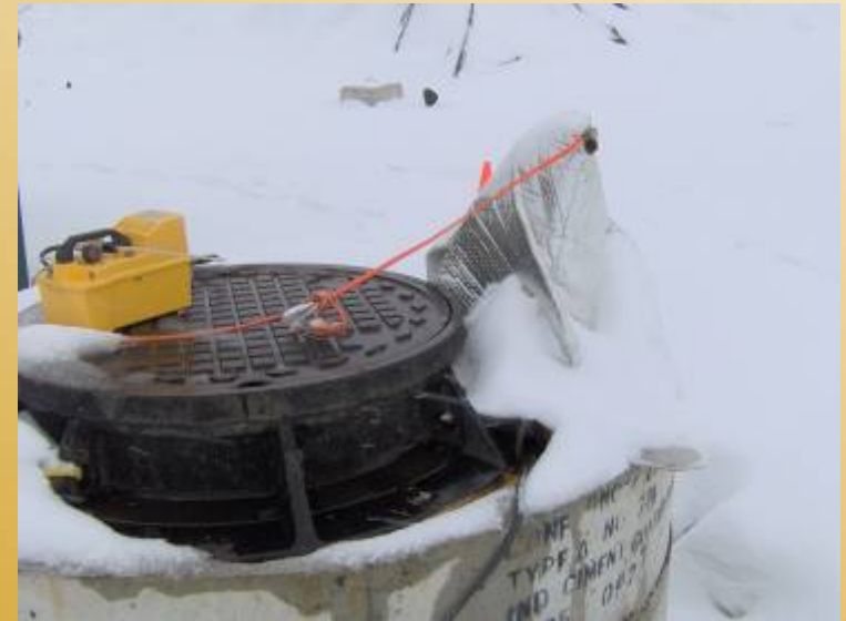
Monitoring of air drawn from the soil
