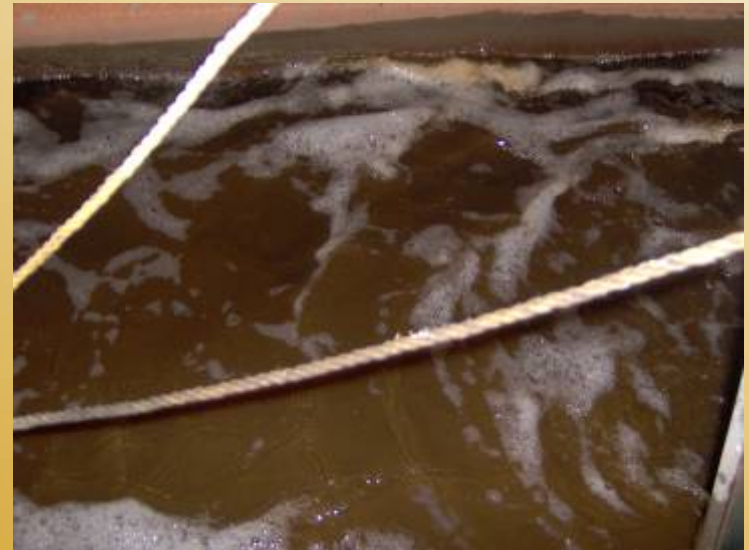
The foam indicates when a batch is ready
