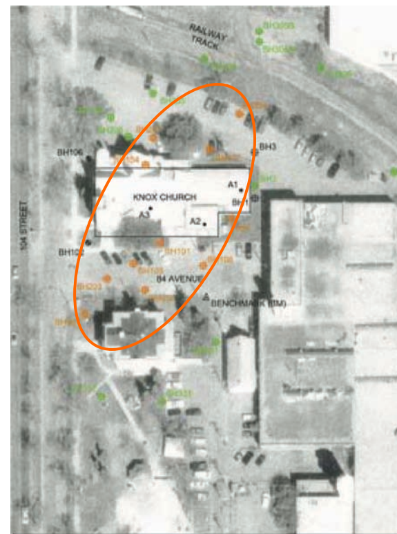
Dissolved Hydrocarbons in Monitoring Wells (Orange)
