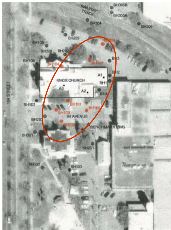
Diesel Fuel Product in Monitoring Wells (Red)
