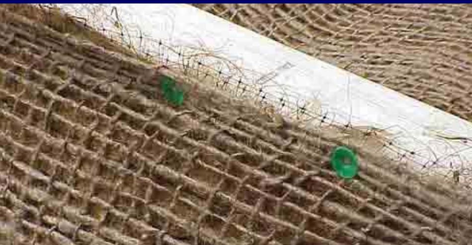
Jute woven mat has most effective adhesive properties for the flocculant
